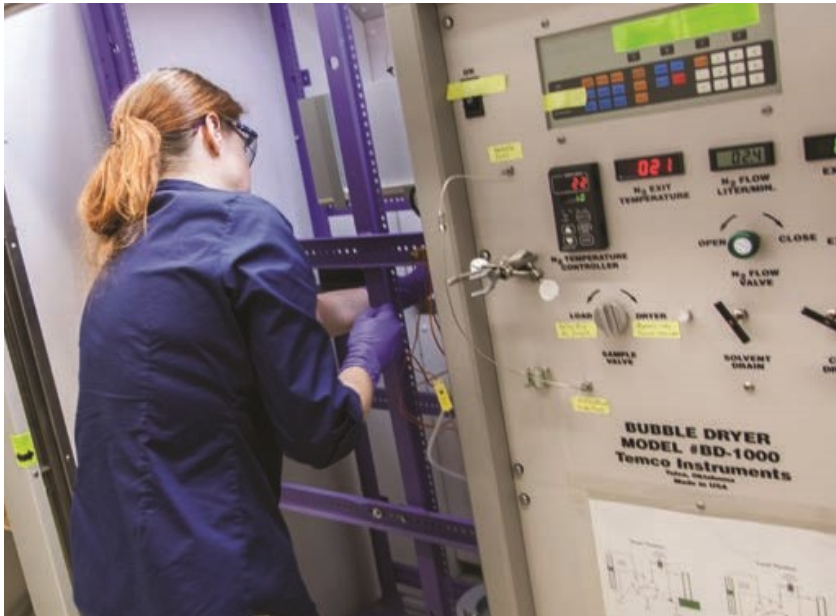
This bubble drier is used to make liquid vaccines into powder by drying micro-sized vaccine particles.
