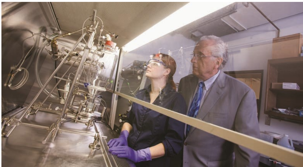
Bob Sievers and a colleague look over the CAN-BD process for making powder vaccines, which involves placing the liquid vaccine under highly concentrated carbon dioxide pressure to form bubbles that repeatedly burst and become smaller and smaller.
