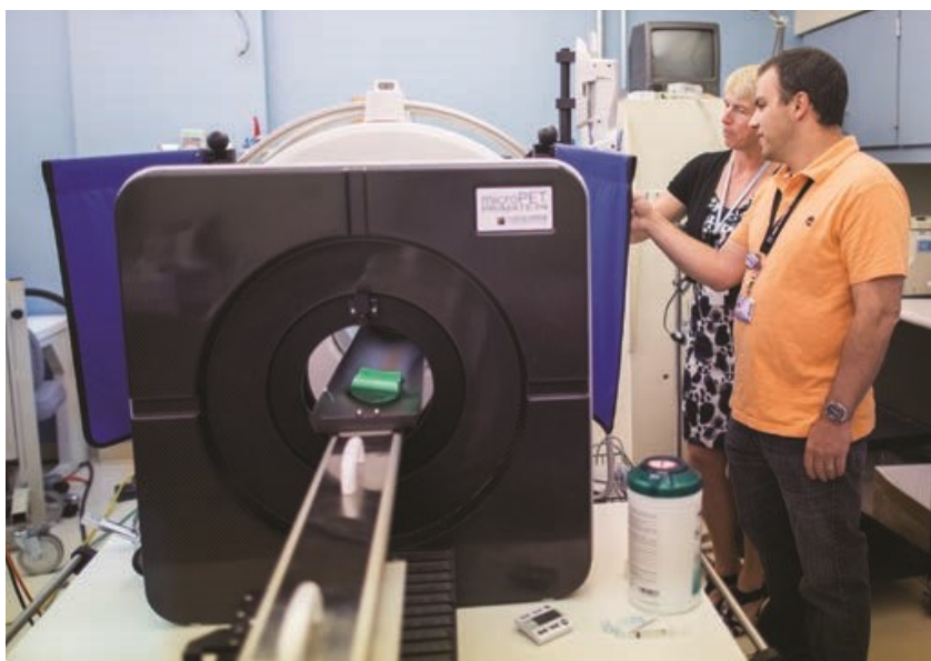
Positron emission tomography (PET) coupled to a computerized tomography (CT) scanner is used to visualize small tuberculosis lesions in the lung, revealing the heterogeneity of the disease.
